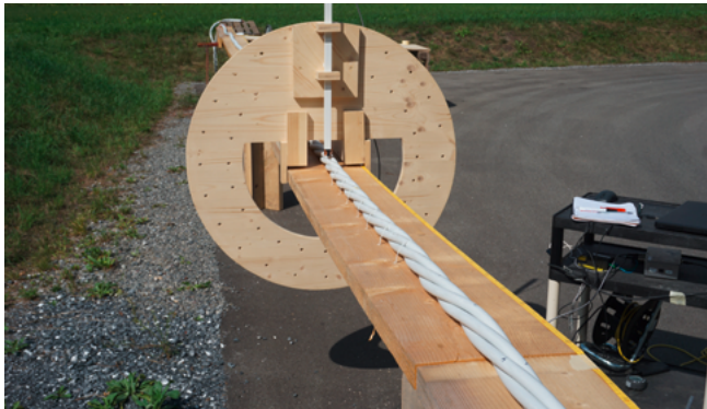
20-meter measuring bench with division apparatus for measuring magnetic fields in the near and far range.
